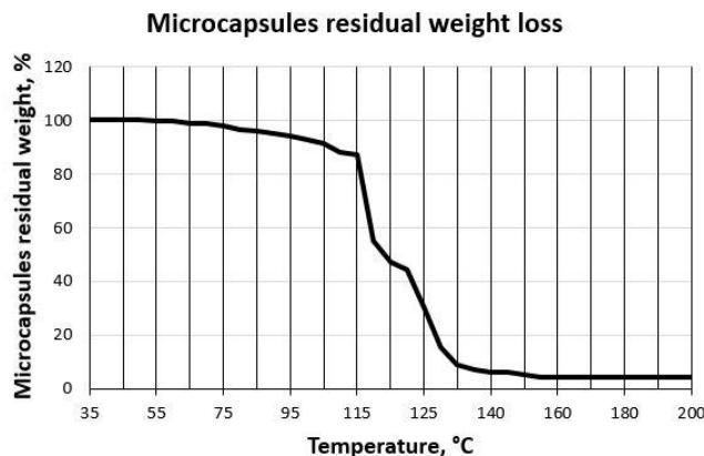
TGA analysis provided demonstrate fluoroketone release rate.
