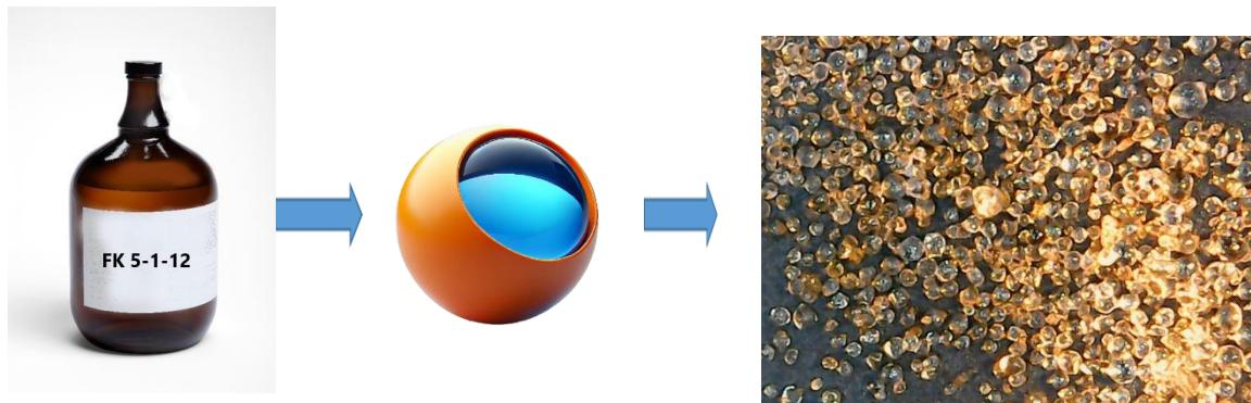
The core of EXTO Technology processing is based on coacervation and emulsion-based methods applied to fluoroketone to put it in polymer shell made of modified gelatin or URF resin + PVA as the main shell materials.
