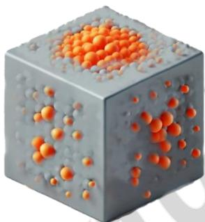
The main microcapsules application technology is its usage as a fill material together with various binding polymers and adhesives (like silicones, synthetic resins, etc.) forming in this combination a thermoreactive applied material. Important limitation – the binder should not be water or acrylic based, as that can damage the microcapsules.
